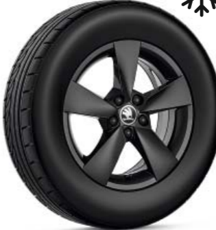
15" HADAR black metallic alloy wheel 5.5J×15" ET40, 185/65 R15
