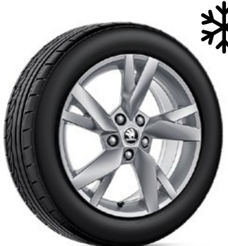
17" LYRA silver alloy wheels* 6.5J x 17" ET46 for 205/55 R17 tyre
